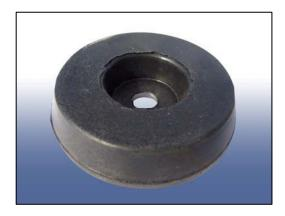
The FPA range of ring mountings are an easy to install method of providing vibration isolation (both active and passive ) together with a measure of shock reduction to a wide variety of applications. Ring mountings consist of a rubber section bonded to a single steel support plate. A clearance hole is positioned in the centre of the ring mount which can also be used with a height adjuster arrangement (not supplied).
